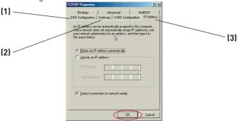
If "Specify an IP address" is selected, your Modem/Router will need to be set up for a static IP connection type. Write the address information in the table below. You will need to enter this information into the Modem/ Router.
